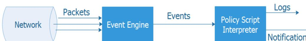
**Figure 2** Architecture of Bro and packet processing flow
